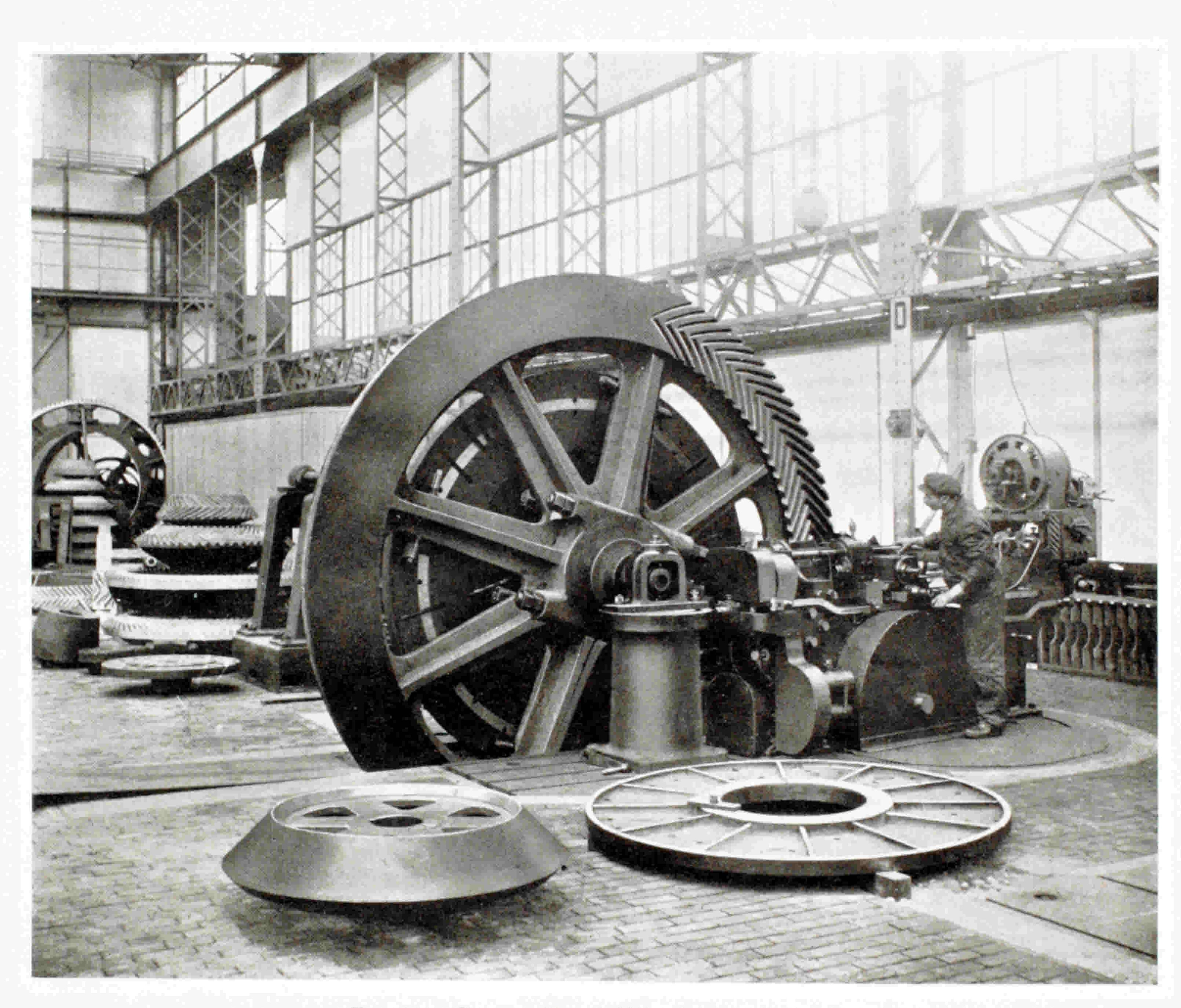
Fig. 2.—Citroën Bevel Wheel partially cut.
