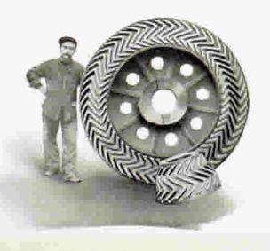
CITROEN DOUBLE HERRINGBONE BEVEL GEARS, as supplied in large quantities for STEERING ENGINES to Messes HARLAND & WOLFF, Ltd.
