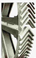
straight-toothed gears, because the joint in the rim of Citroen Gears has the exact shape of a double helical rooth, which causes the two halves to interlock. Thus the strain on the assembling bolts, which is so prominent in straight-toothed Spur Gears, is greatly relieved in the case of Citroen Gears.
