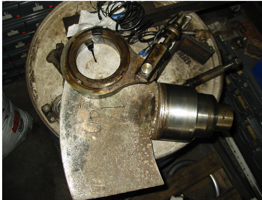
Close up of freshly removed blade, bell crank and tie rod.
