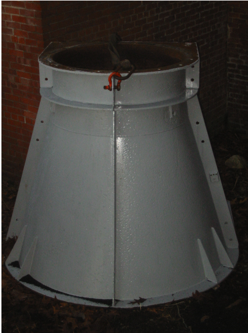
This is the outer cone. The inner cone is attached to this cone by an angle iron frame on the discharge end and three, tensioned, spokes on the propellor end.
