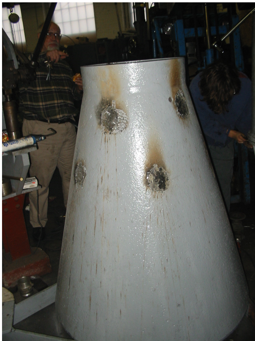
Patches welded in place.
